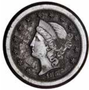
Fig. 26: United States: California. Kellogg & Co. private coinage, steel obverse hub for 20 dollar gold coin die, 1854-5 (without last digit added). Hub of Kagin 1-3, Breen 7917-20, Friedberg 37. (ANS 1921.136.4, gift of Anita P. L. Kellogg) Diam. of hub base 40 mm, diam. of hub face 32 mm, height 41 mm.
