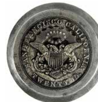
Fig. 25: United States: California. Kellogg & Co. private coinage, steel reverse hub for 20 dollar gold coin, 1854-5. Hub of Kagin 1-3, Breen 7917-20, Friedberg 37 (ANS 1921.136.5, gift of Anita P. L. Kellogg, daughter in law of the coiner John Glover Kellogg) Diam. of hub base 45 mm, diam. of hub face 32 mm, height 39 mm.
