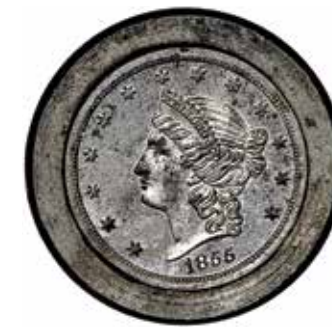
Fig. 24: United States: California. Kellogg & Co. private coinage, steel obverse die for 20 dollar gold coin, 1855. Breen 7920; Kagin 3b (ANS 1921.136.2, gift of Anita P. L. Kellogg, daughter in law of the coiner John Glover Kellogg) Diam. of die base 46 mm, diam. of die face 32 mm, height 49 mm.
